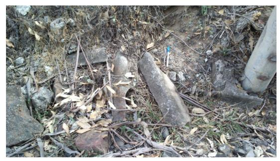
PHOTOGRAPH 9 Corrugated fibrous cement sheeting within the loading ramp – central west portion of Area 4. (Sample 404-3 collected).
